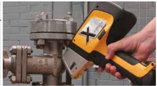
**PMI Equipment.** A new generation of Positive Material Identification Equipment gives WALWORTH the capability to perform quick chemical analysis on incoming raw materials and on pieces after assembly, to certify that materials used were produced and assembled in accordance with WALWORTH's and our Customer's specifications.
