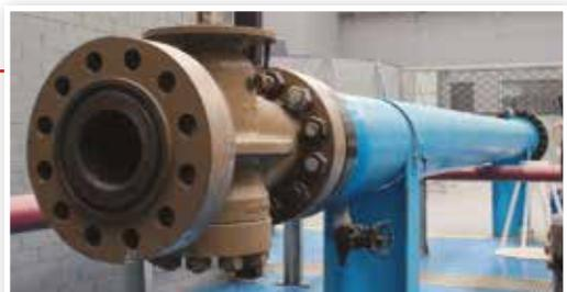
**Pressure Gradient Test Loop.** This test exposes Plug valves to the extremes of both positive and negative pressure gradients to verify that the plug in a balanced plug design will prevent lock-up in the body.
