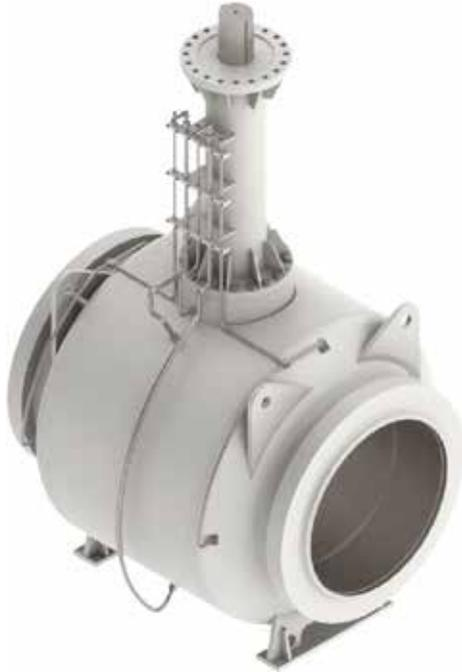
There are pipe systems that run underground thus, buried valves that are not easy to reach and operate do require stem extension to facilitate access. This improvement is also recommended for services under extreme temperatures such as - 50°C or lower and 220°C or higher.
