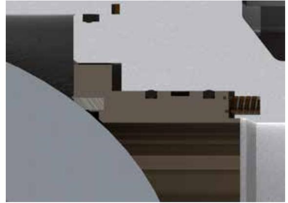
Spring loaded seats achieve low operating torque at different positions under high working pressures. Each seat ring is placed at each end of the ball in a way that the components achieve alignment whenever the valve is fully opened; the rings are pushed towards the obturator by a set of coil springs which ensure appropriate sealing at low pressure before piston action effect takes place.
