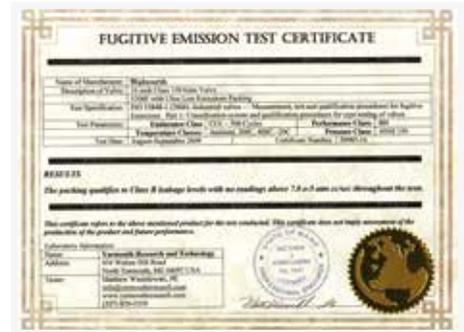
**Emissions after 500 cycles at ambient and 350 °F Issued by Yarmouth Research and Technology Lab for 16 inch Class 150 Gate Valve After 500 cycles the measurement result was less than 50 ppm.**
