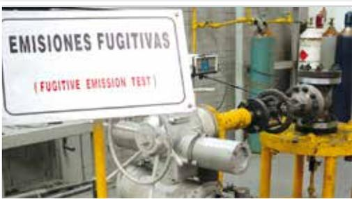
**Low Fugitive Emissions Test.** This test is performed when a Customer requires low fugitive emissions certification. Our Lab has its own LFE test equipment that is capable of measuring less than 20 ppm in both static and mechanical conditions at either ambient temperature or thermal cycle operations.
