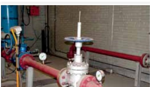
**Test Loop.** A complete Laboratory Test loop exists for design validation of WALWORTH products. The test is performed at maximum design pressure, advances the valves from 3000 to 5000 cycles, and requires more than four months to complete.
