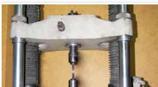
**Tensile Test Equipment.** We use this equipment to verify the mechanical properties of materials used for manufacturing. WALWORTH tests samples on a random basis even though we receive MTRs from our suppliers and foundries.
